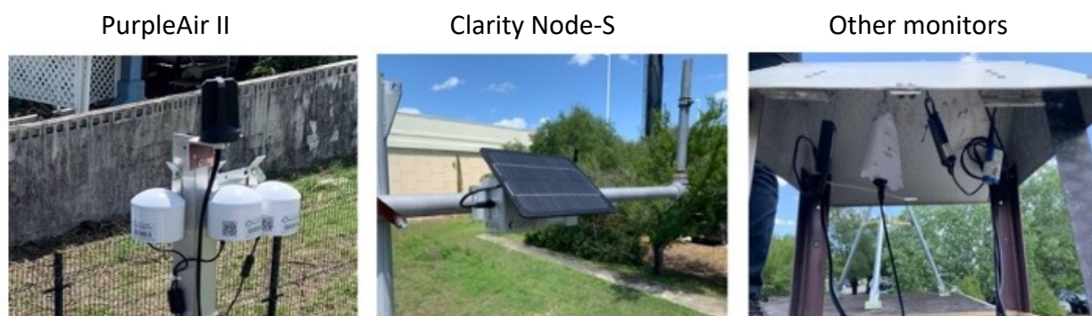
Figure 1. Images of co-location installations of the candidate low-cost monitors. The additional monitors shown in the rightmost image are the Atmotube Pro, AirBeam 2, Flow2, and Cairsens (from left to right).
