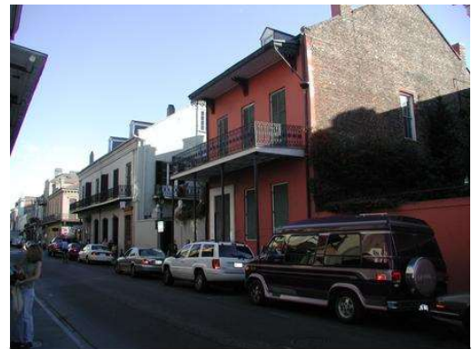
Streets, like the one pictured, are narrow enough to discourage speeding but wide enough to allow on-street parking.
