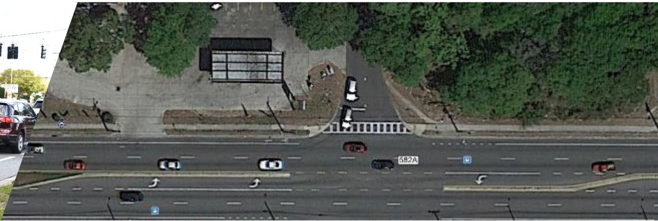
Added Raised Traffic Separators
