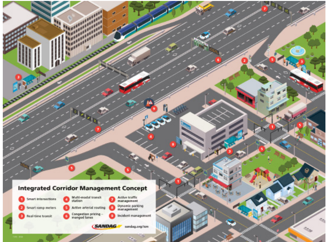
An innovative solution to congestion is planned for I-4. This corridor will be instrumented with technology to proactively inform users of traffic jams and quickly deploy resources to clear incidents.
