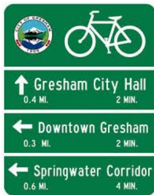
Figure 2-10: An example of a bicycle route sign used in Gresham, OR that includes distances to destinations and identifies to roadway as a bicycle boulevard
