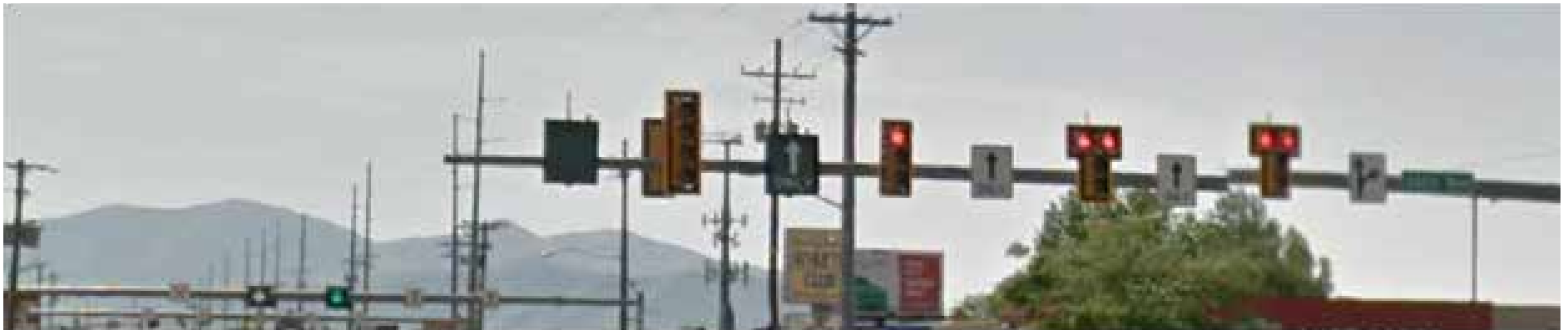
Figure 13. Reversible Lanes Signalized Intersection Hardware Example
