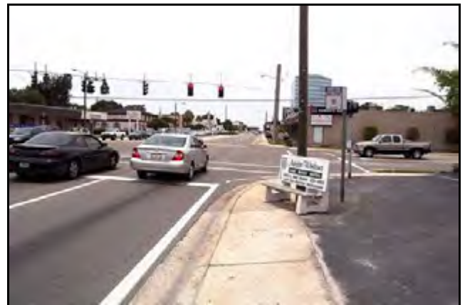
Figure 3-4 Example of Sidewalk Obstructed by Bench
