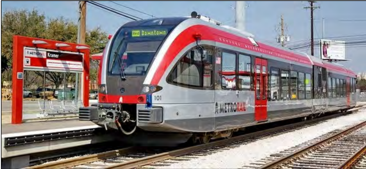
The Capital Metro MetroRail Red Line, which operates between Leander and Downtown Austin, Texas, is an example of a DMU Commuter Rail service.
