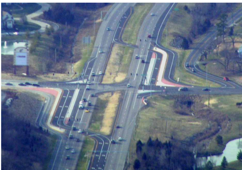
Figure 2.5: Continuous Flow Intersection in Fenton, MO
