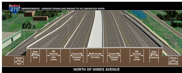
Figure 3. FDOT Proposed Typical I-275 Cross-Section
