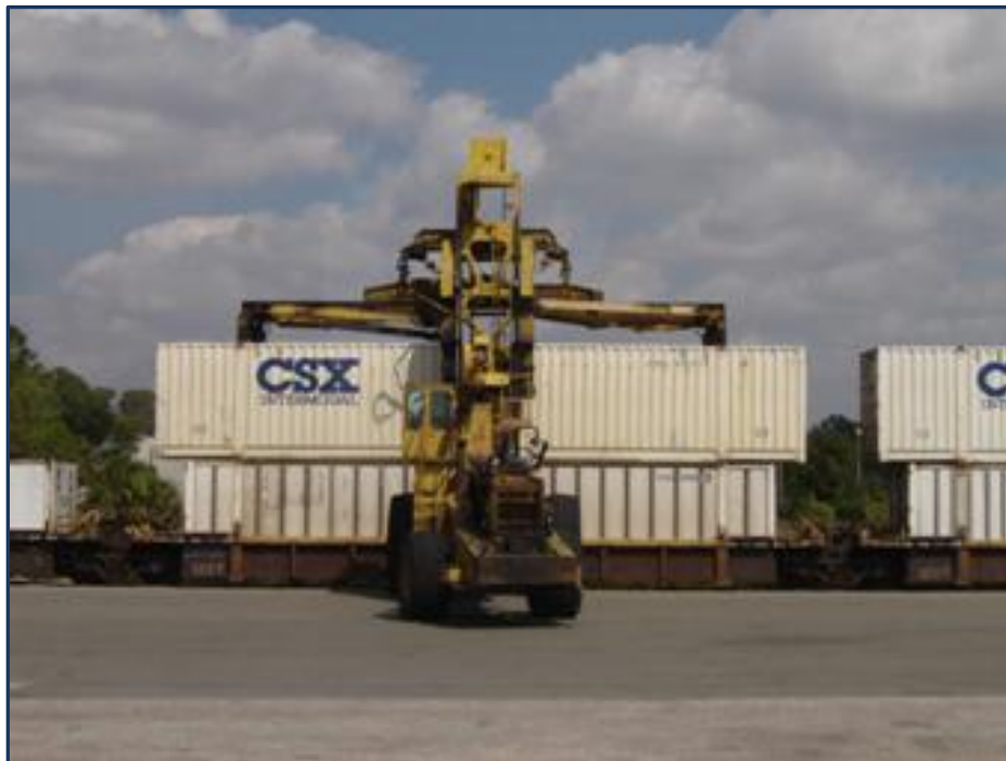
Double-stacking a 53-foot domestic container onto a rail intermodal car at the Tampa CSXI Terminal.
