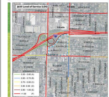
Source: Tampa Bay Regional Planning Model (TBPRM) 2035 Highway Network Volume to Capacity ratios
