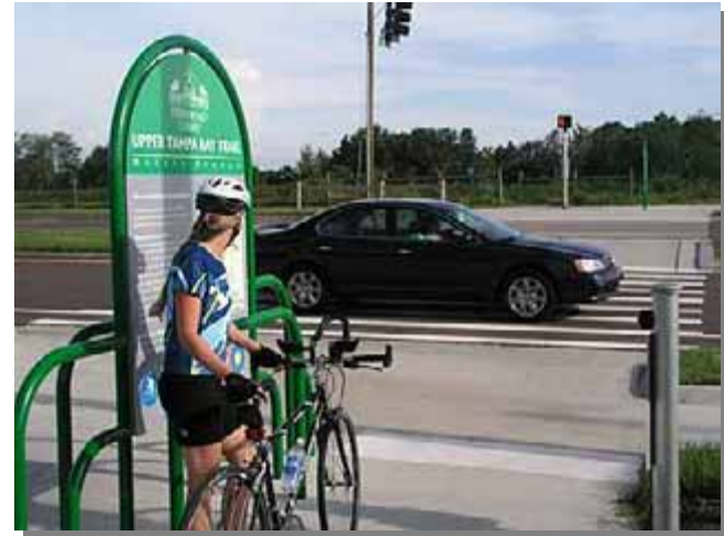
Figure 2.7: Minimize the number of times trails must cross roadways or driveways
