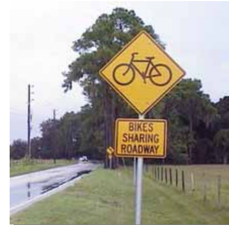
Figure 2.25: Where bicyclists and motorists share roadway, signs should be posted alerting motorists
