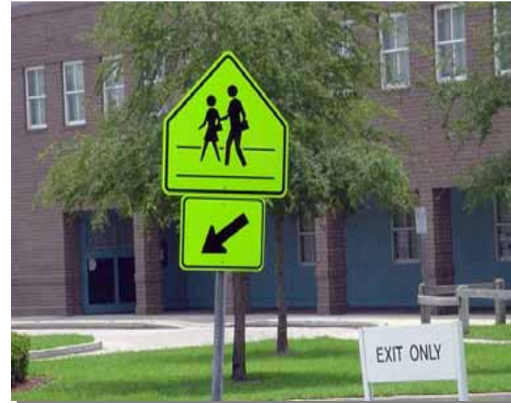
Figure 2.44: Multiple pedestrian crossing signs may be necessary in areas of high pedestrian traffic, such as near schools
