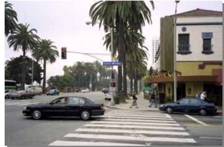
Figure 2.11: Ladder style crosswalk markings
