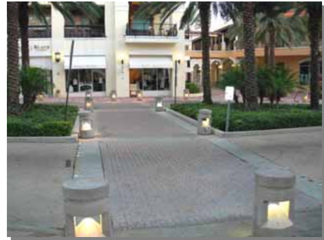
Figure 2.28: Bollards and specialty paving are used to define this pedestrian crossing
