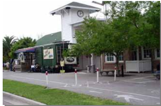
Figure 2.8: Bollards should be used to deter vehicular use of multi-use trails
